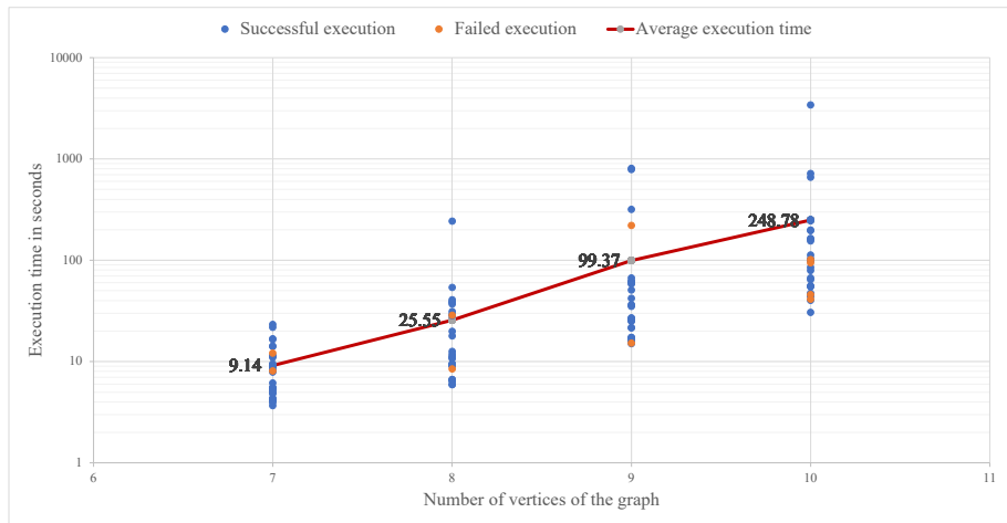
FIGURE: Results of running the greedy optimization algorithm on 120 random graphs with different numbers of vertices n where each edge appears in the graph with probability 0.2. Thirty graphs were tested for each n . From left to right, the success rates are 0.93, 0.93, 0.93 and 0.87.
