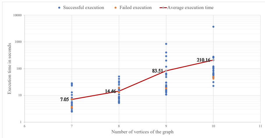
FIGURE: Results of running the greedy optimization algorithm on 120 random graphs with different numbers of vertices n where each edge appears in the graph with probability 0.3. Thirty graphs were tested for each n . From left to right, the success rates are 0.90, 0.93, 0.97 and 0.93.
